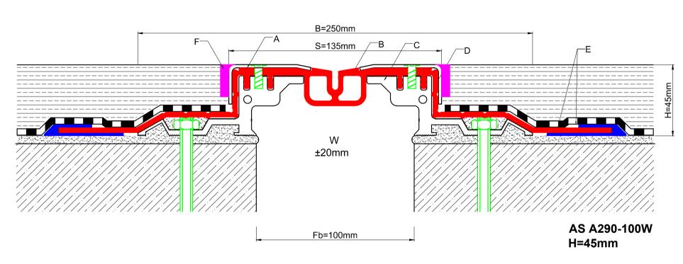
A Stainless steell cover 2mm B Replaceable EPDM insert
